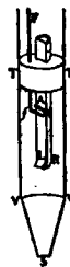
FIG. 2.—Organ pipe fitted with beating reed. AL, Beating reed. R, Reed box. F, Tuning wire. TV, Feed pipe. VV, Conical foot. S, Hole through which compressed air is fed.
